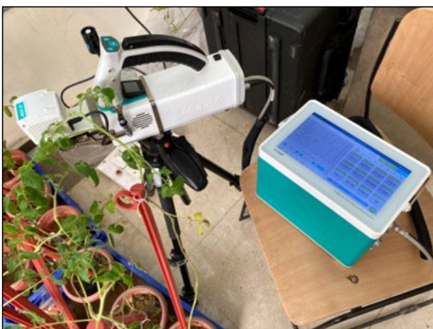
Figure 3: The IRGALI-6400XT Portable Photosynthesis System used to record physiological parameters of tomato plant
